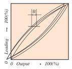
The ability of a load cell to reproduce output readings when the same load is applied to it consecutively, under the same conditions, and in the same direc-tion. Repeatability is expressed as the maximum difference between output readings as a percent of rated output.
